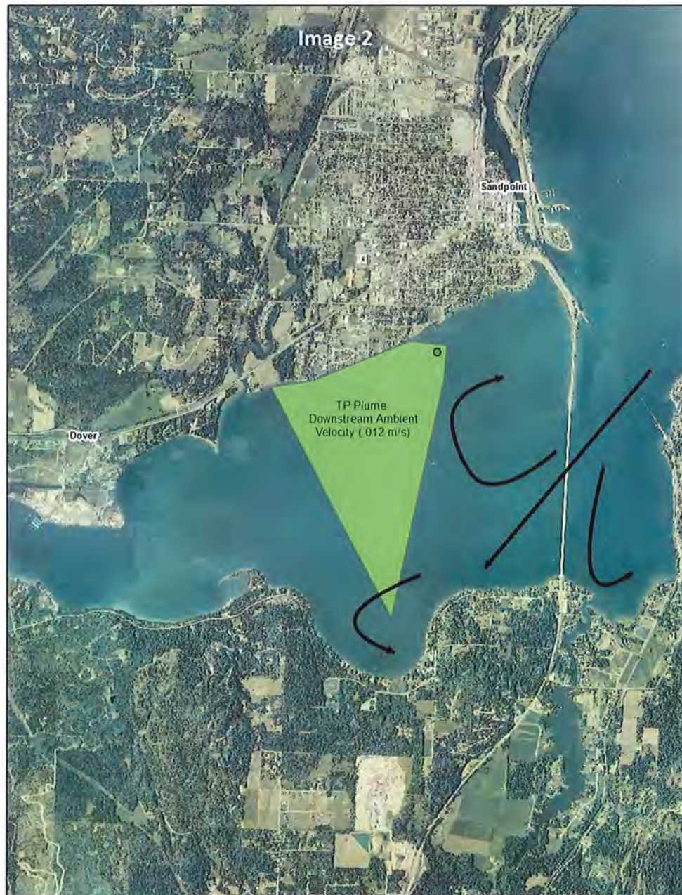
Image 2 Early CORMIX Modeling Scenario Phosphorus Concentration of 2867 \mu g/L; Facility Design Flow of 3.62mgd and River Flow of 8,448cfs
